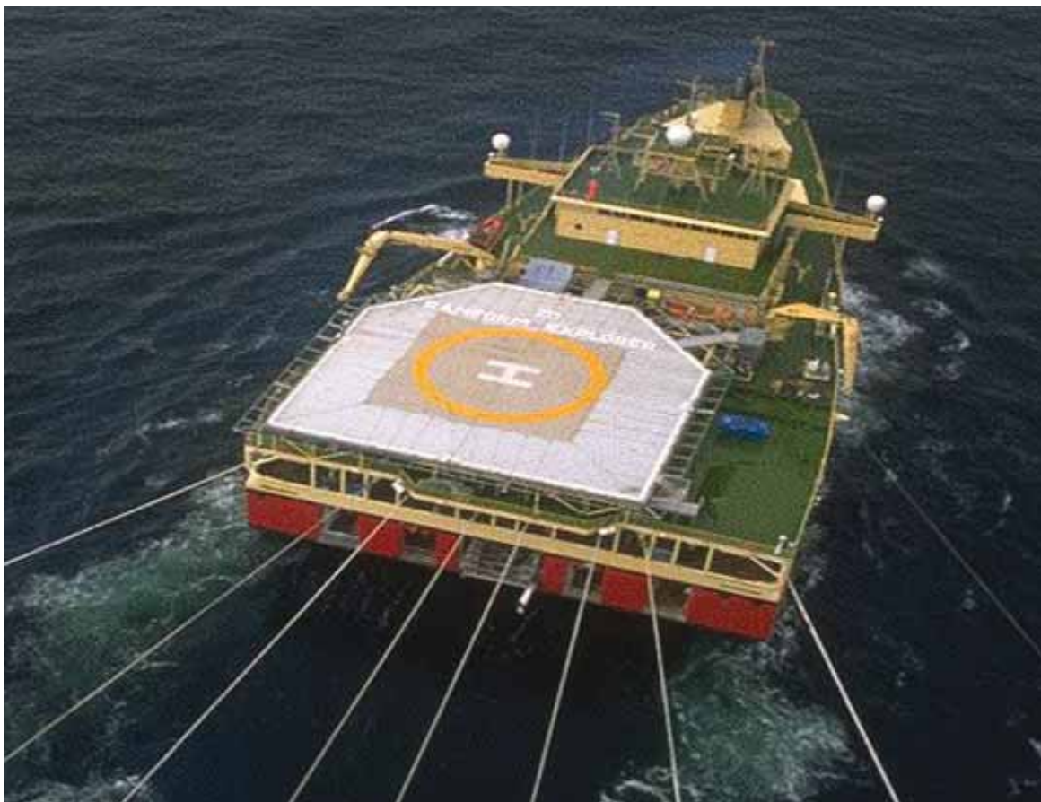
Seismic vessel towing streamers that emit signals and map the subsurface
